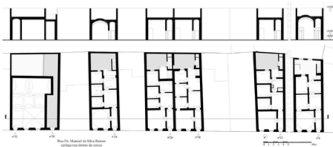
12. Façade, section and plans of a set of houses with different types located in standard lots in the former Rua de trás das Cercas (current Rua Dr. Manuel da Silva Ramos) in Fuzeta. (Author's drawing)
